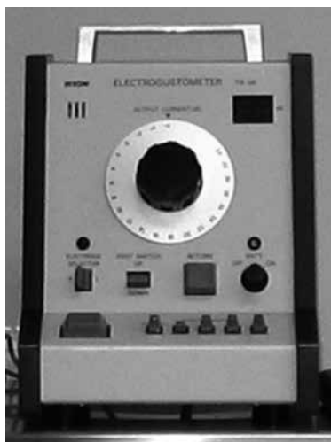
Figure 2 The electrogustometer(TR-06 model, Rion Inc.,Tokyo) was used for electrogustometry.
